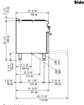
El = Electrical inlet (power)EQ = Equipotential screw
